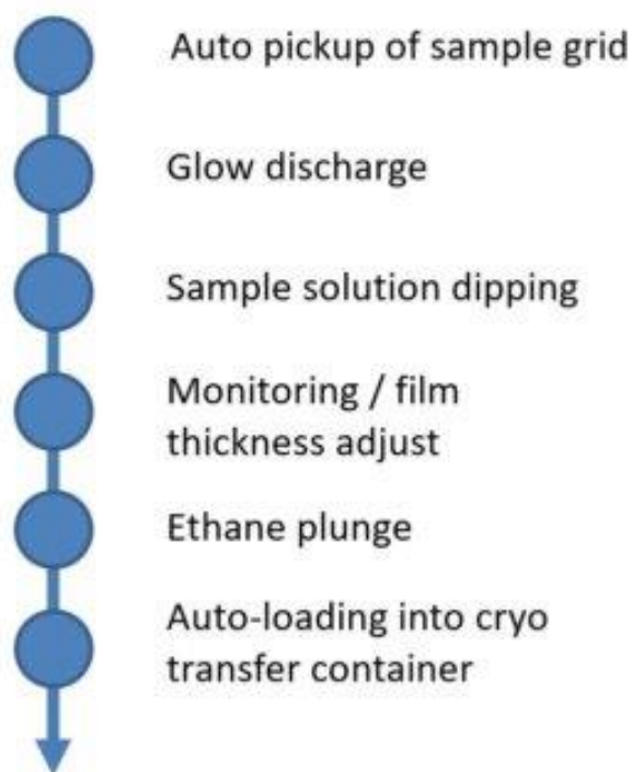
Figure 2. Typical automated sequence for the preparation of cryo-samples on an EM grid in the automated plunger system.
