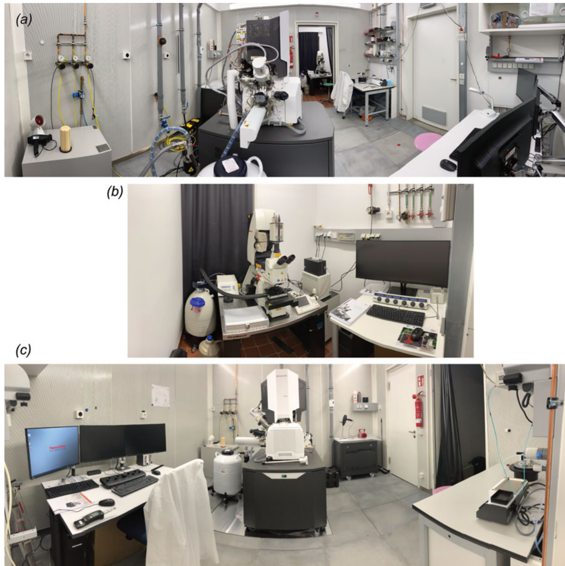
Fig. 3. Room for CLEM. (a) Aquilos cryo-FIB-SEM (TFS) with Leica SP8 confocal cryo-CLEM in the background. (b) Close-up of the cryo-CLEM. (c) Front view of the Aquilos FIB-SEM.
