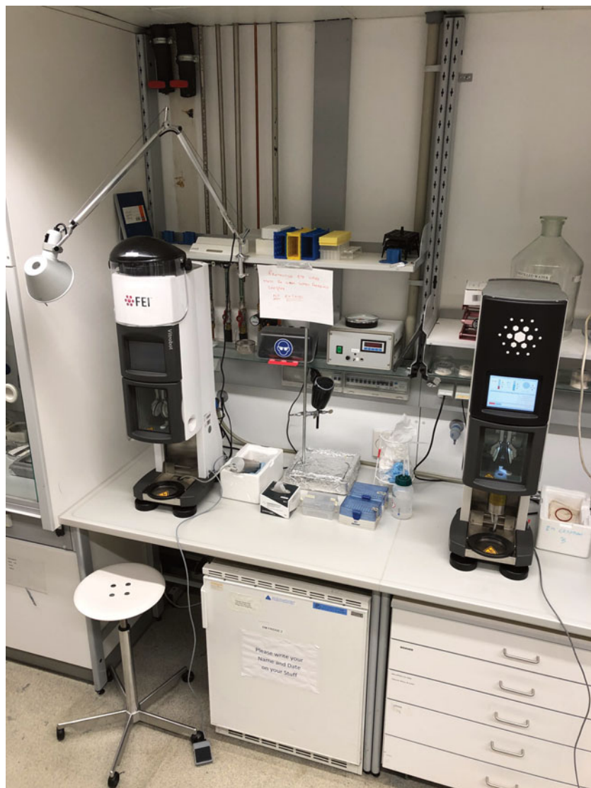
Fig. 4. Vitrification robots. Two different Vitrobot models from TFS.
