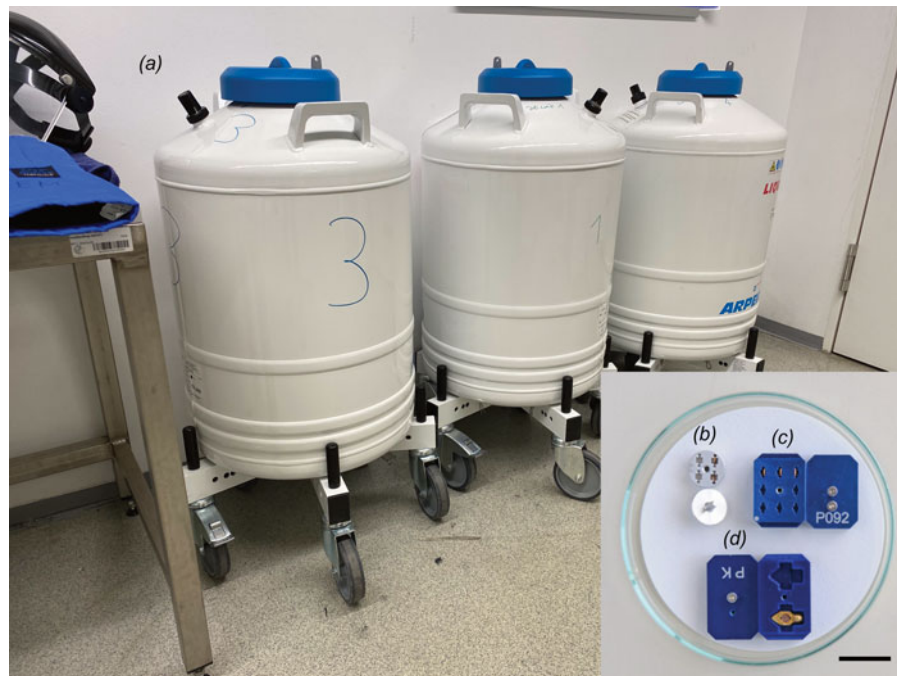
Fig. 5. Storage of cryo-grids. (a) Storage Dewars. Inset: Grid storage boxes. (b) Commercially available plastic, four-slot box for cryo-grids or Krios specimen cartridge (TFS). (c) Custom-designed eight-slot aluminium box for cryo-grids or Krios cartridges with identifying number. (d) Custom-designed two-slot aluminium box for Polara cartridge with identifying number. Scale bar: 2 cm.
