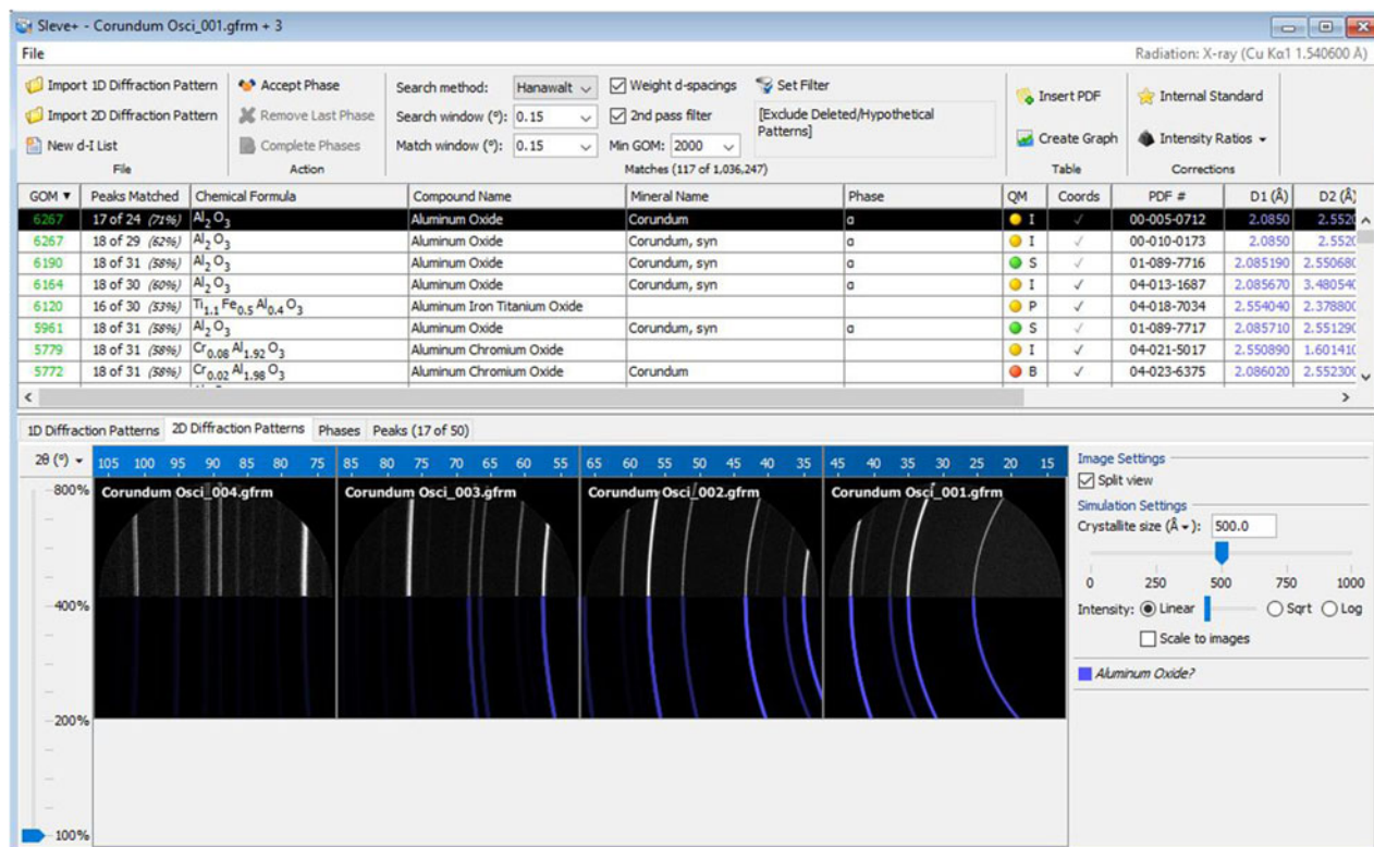
Figure 14. Example of phase identification using 2D diffraction data.
