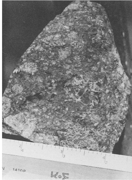
Fig. 6. Fresh rhyolitic breccia with spherulitic lithic fragments, and whole and fragmental spherulites in the matrix.
