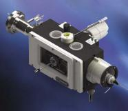
The PP3010T is a highly automated, easy-to-use, column-mounted, gas-cooled cryo preparation system suitable for most makes and models of SEM, FE-SEM and FIB/SEM. The PP3010T has all the facilities needed to rapidly freeze, process and transfer specimens.
