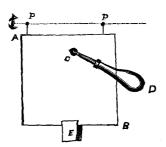
A B is a square piece of board,—accuracy of form is immaterial. It may be of any size, say six inches square. E is a piece of lead, bent so as to embrace the lower edge, and capable of being made to slide tightly along it. D is an awl passing loosely through a hole at C. P P are two common pins, stuck into the upper edge of the board.
