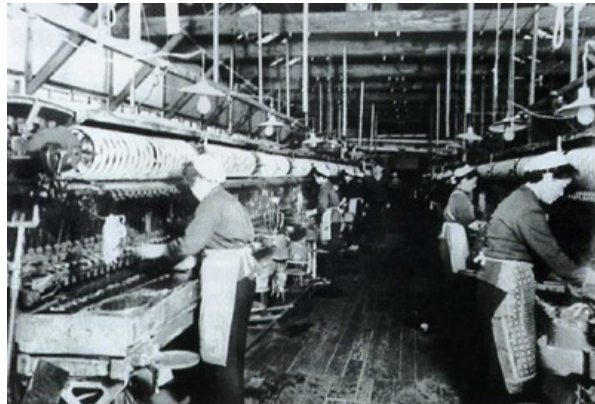
Female factory workers at a textile factory using Masuzawa-style reeling machines, similar to Minorikawa-style. Source.
