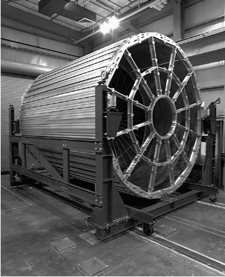
Figure 10.14 Field cage support structure of the STAR TPC at RHIC. Picture courtesy Brookhaven National Laboratory (USA).
