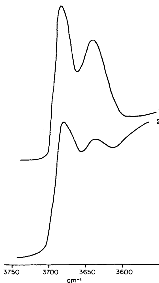
Fig. 7. Mg-V. Structural OH spectra (1: hydrated- 2: heated to 250°C under vacuum).
