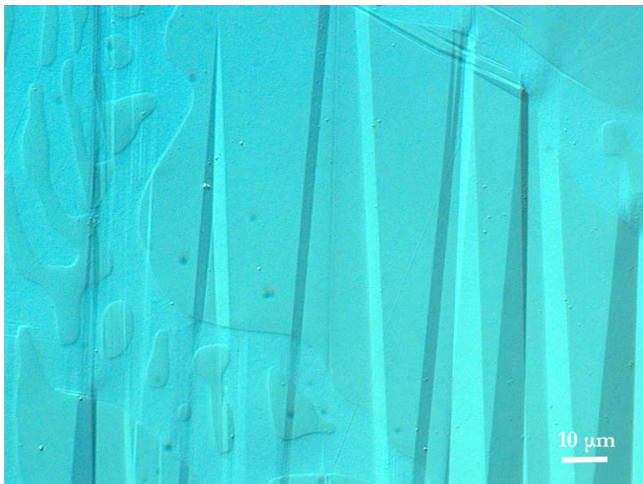
Figure 1. Lamellae of L 10 martensite stabilized at room temperature by A1 particles in B2 matrix of the annealed and quenched Co 38 Ni 133 Al 29 alloy. The example shows the structure investigated for stress induced lamellae interaction with A1 precipitates.
