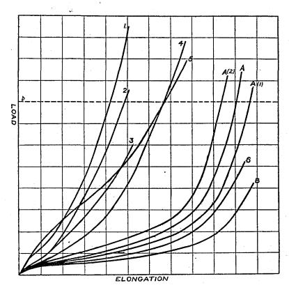
Dr. Geer, of the Goodrich Rubber Co., has described a series of ageing tests for rubber. These or similar tests are universally used. He was the first to describe them in detail. The method consists in testing portions of the rubber and then ageing other pieces in an electric oven kept at 700° Cent. or thereabouts. After which the tests are applied and the difference in the figures is a measure of the deterioration produced.
