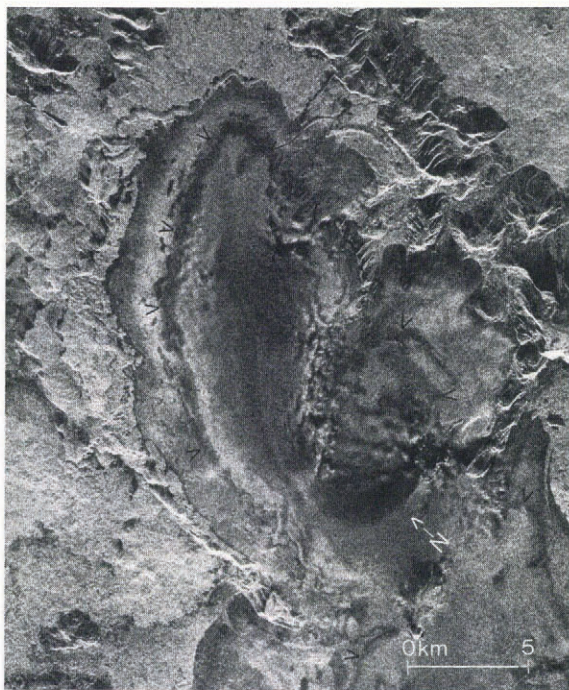
Fig.4. Part of Seasat SAR image of Iceland acquired on 24 August 1978, showing the northern part of the Langjökull ice cap, processed at DFVLR, Oberpfaffenhofen, Germany. SAR look direction is from bottom to top. The black arrows point to the snowline on the glacier.
