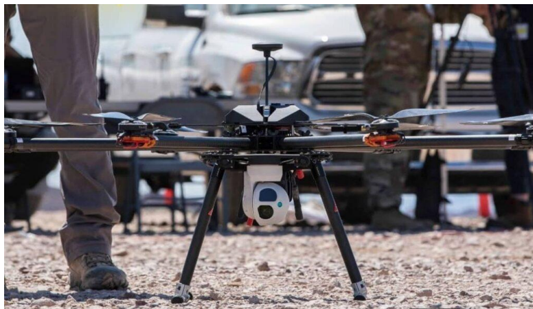
Figure 1. The Robotic Autonomous Platform for Tactical Operations and Reconnaissance (RAPTOR) unmanned aerial vehicle (UAV)
