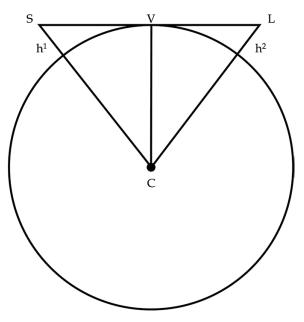
Fig. 11. Visibility calculation based on the curvature of the earth. S represents the sailor, with h1 as the sailor's eye level; L represents the lighthouse, with h2 as the height of the lighthouse light. C represents the centre of the earth, and V represents the place on the horizon after which the lighthouse would no longer be visible.
