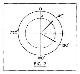
If the pilot were able to see this last diagram he could deduce from it his bearing relative to the scan axis, and make the necessary flight corrections (assuming he knew his aircraft heading)
