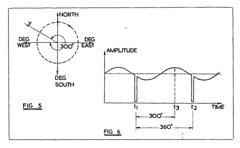
The ultimate object of the system is to guide a helicopter down the vertical axis OX If a helicopter is situated somewhere off this axis at Y' then a suitable receiver in an aircraft would receive a fluctuating signal. The signal would be maximum when the beam is to the right and of magnitude proportional to OA and the minimum when the beam is to the left, and of magnitude proportional to OB, thus the output of the receiver would be of the form shown in Fig 3
