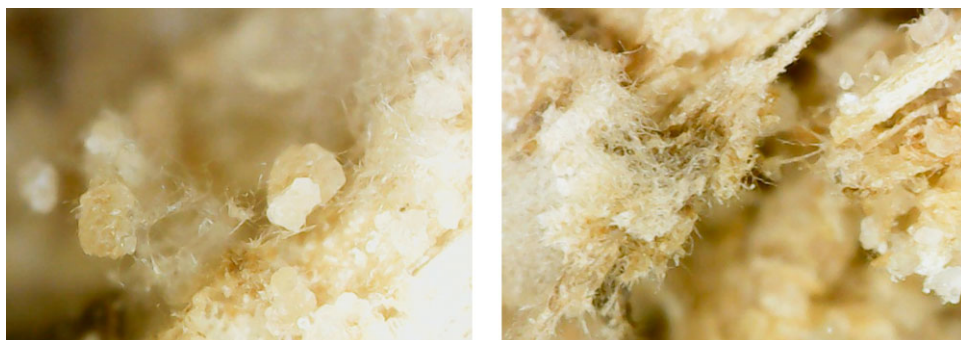
Figure 5. Calcite formation on mycelium network interior of an MBBC sample, magnification approx. 800 with a digital microscope, after 5 days of cementation solution submersion and multiple days of drying.
