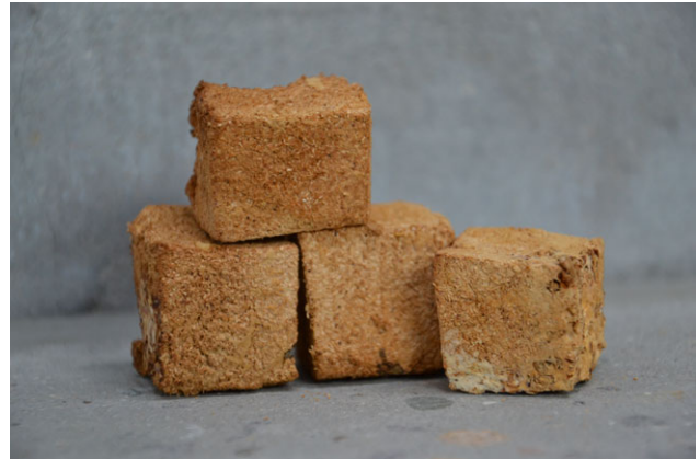
Figure 14. 3 \times 3 \times 3 cm cubes of MBBC after biocementation and drying at room temperature.
