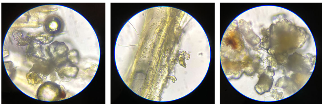
Figure 6. \text{CaCO}_3 formations on and around mycelium and wood substrate, light microscope, 1000 \times magnification.
