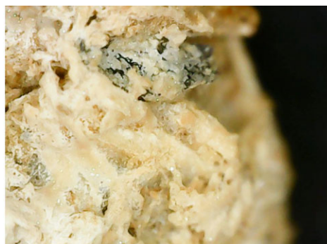
Figure 2. Different sized accumulations of \text{CaCO}_3 in between and attached to mycelium, light microscope 1000× magnification.
