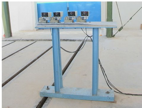
Figure 12. The speedometer sensors which measured the speed of bird in bird impact experiment.
