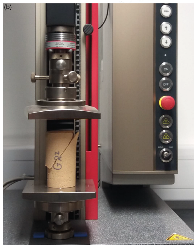
Fig. 5. Mechanical testers used in this study: (a) ring-shear tester sketch (modified after Schulze, 1994) and (b) uniaxial compression tester.
