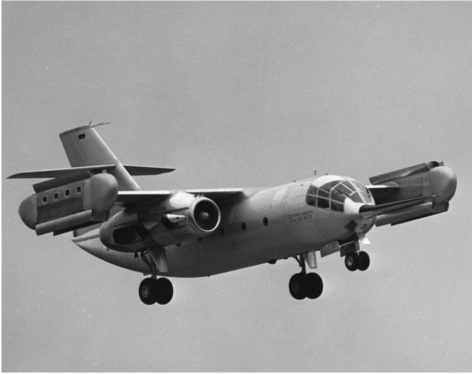
Figure 27. The unusual Dornier Do 31 had no less than eight RB.162 lift jets housed in the outer nacelles.
