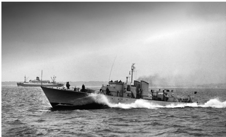
Figure 31. The RM60 gas turbine enabled the HMS Grey Goose to reach speeds in excess of 35-kn.
