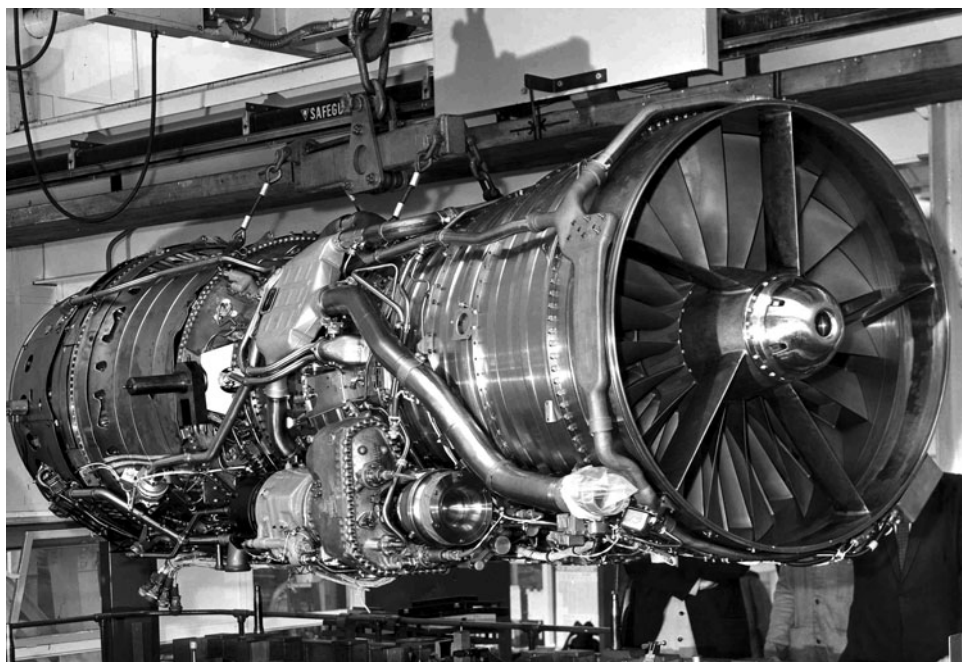
Figure 24. The Olympus proved an outstanding match to the Concorde.
