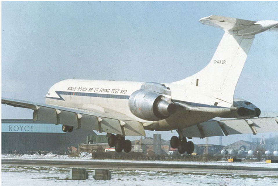
Figure 17. The Rolls-Royce VC10 Flying Testbed, with one prototype RB.211 replacing two Conways.
