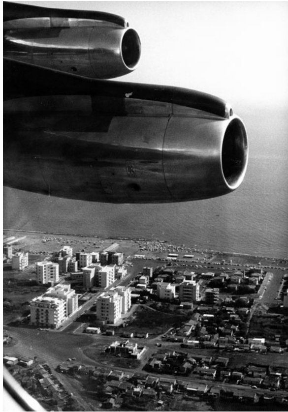
Figure 16. Conways fitted to an Air India Boeing 707.
