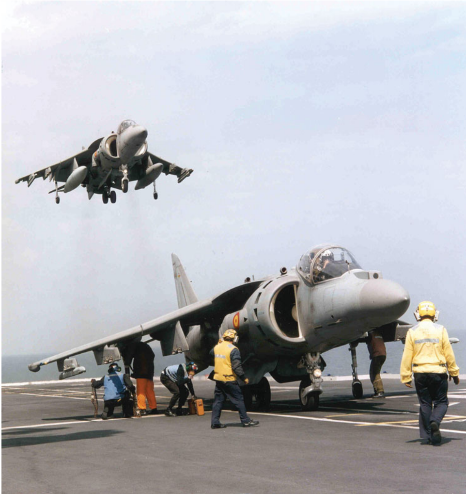
Figure 28. The Harrier required a large inlet to accommodate the huge volume of air sucked in by the Pegasus's fan.
