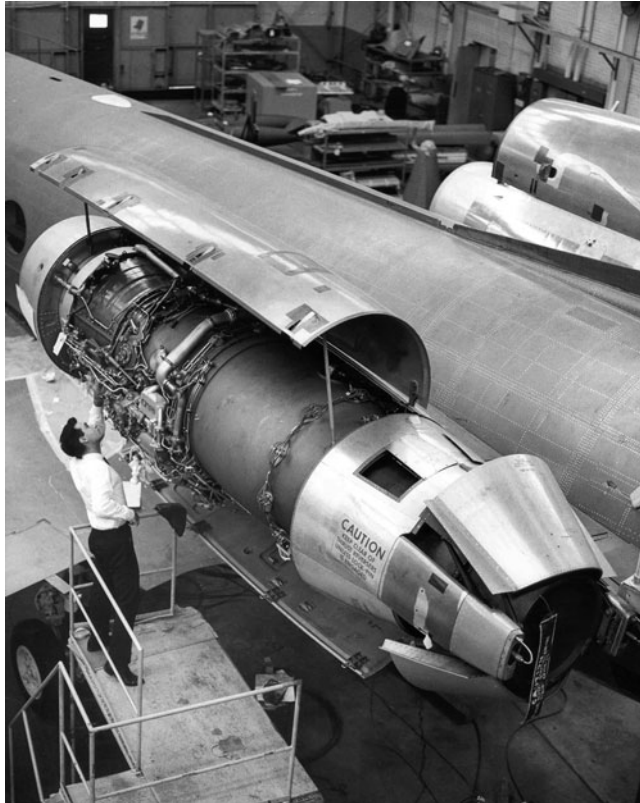
Figure 21. A Spey undergoing installation on a Grumman Gulfstream II.
