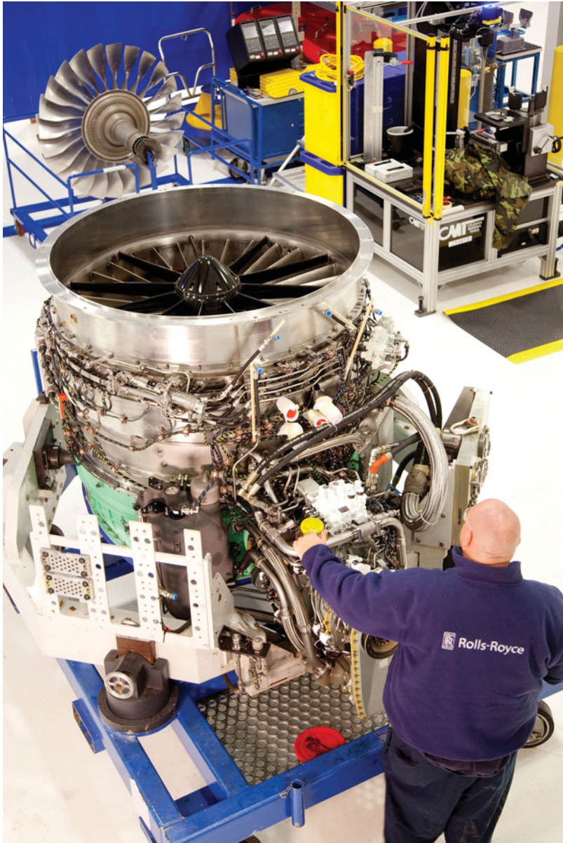
Figure 30. The two-stage, contra-rotating LiftFan ® provides vertical lift for the F-35B.
