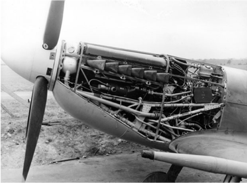
Figure 8. A Rolls-Royce Merlin fitted to a Mk IX Spitfire.
