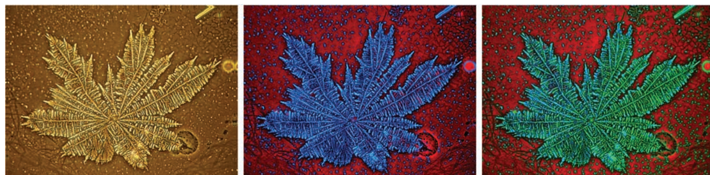
Fig. 10: Hydro soluble pigment, thin-layer crystallization, phase contrast, white light image, bicolor sandwich (monochromatic red and blue light), tricolor sandwich (monochromatic red, green and blue light), objective 40x, ocular 10x, HFW: 250 \mu m
