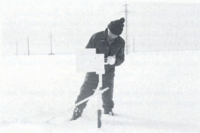
Fig. 6. Cyclone-type drift collector equipped with wind vane.
