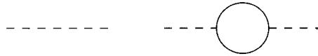
Fig. 4.1. The first two orders in the expansion of the \phi -propagator described by Feynman diagrams in the simple g\phi:\psi^2 -theory. Solid (broken) lines correspond to \psi - ( \phi -)propagators.
