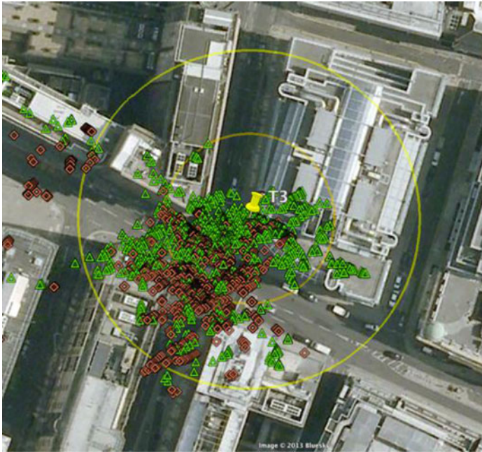
Figure 6. Position solutions for site T3 from Test Set 1. Red diamonds denote conventional elevation-based weighting without height aiding or consistency checking. Green triangles denote a combination of C/N_0 -based measurement weighting, height aiding and consistency checking using subset comparison. The yellow pin in each picture indicates the true position and the circles mark position errors of 25 m and 50 m.
