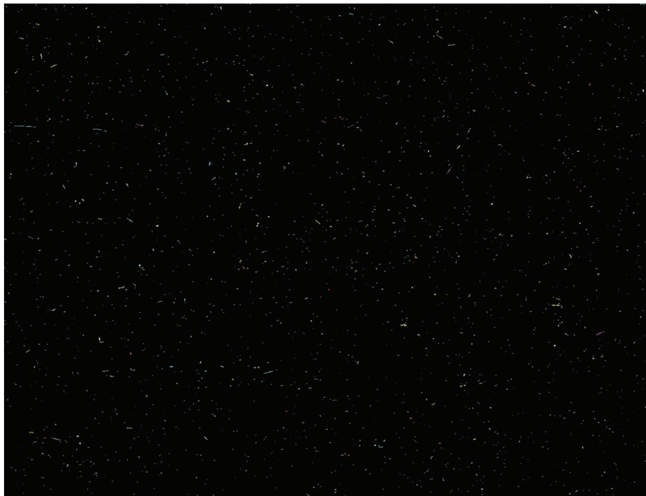
Figure 1: Cosmic ray particle tracks revealed in a five-day-long exposure. Color image combines red 001–180, green 181–360, and blue 361–538 planes into a contrasted 24-bit.tif image.
