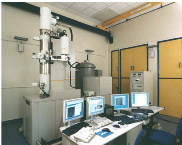
FIG. 1. JEOL JEM-2200FS double aberration corrected 200kV FEG(S)TEM installed in Oxford
