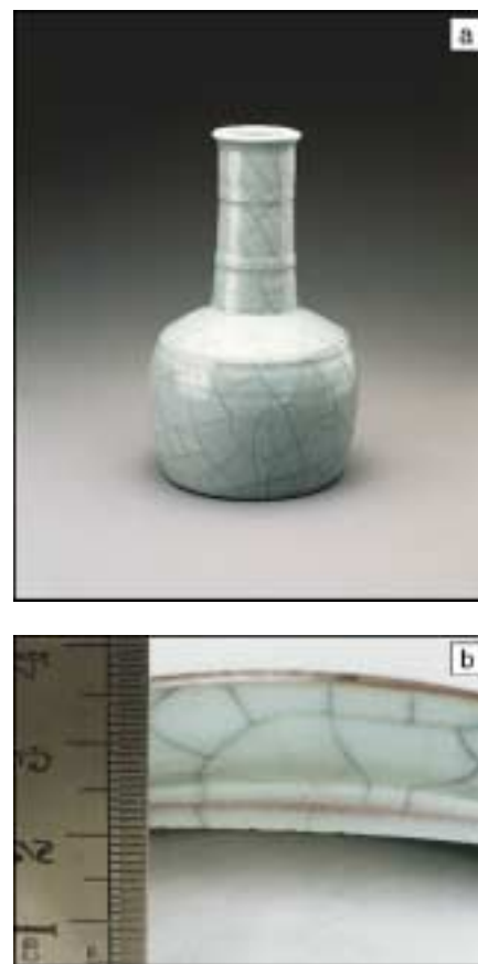
Figure 1. (a) Example of Guan ware (height: 25 cm). (b) Cross section of Guan ware sherd showing thin gray body, thick green glaze, and two-color crackle pattern called "iron wire and golden thread" (From Reference 5). Size marker is in centimeters.
