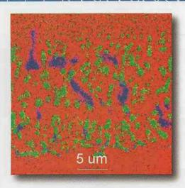
RGB overlay of COMPASS components (256 x 256 pixels) over a SEM image and corresponding spectra with coordinated RGB colors.
