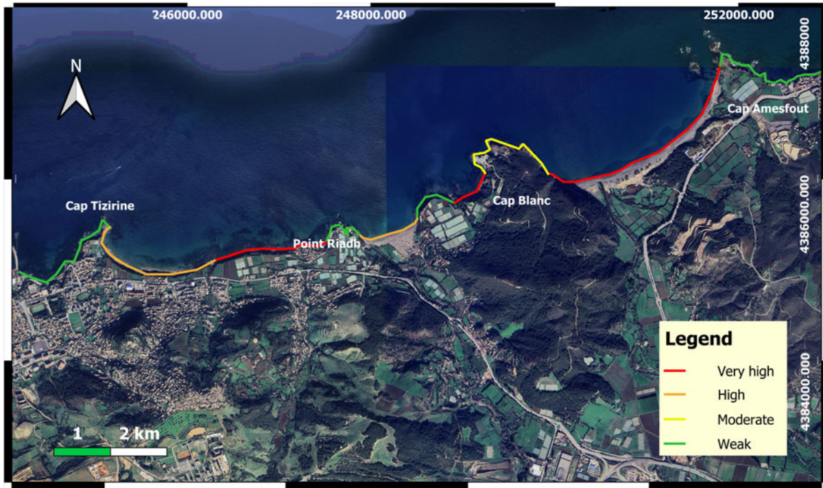
Figure 7. Coastal vulnerability index (IVCphy) for the littoral of Cherchell, after the model of Amrani and Fernane 2021 (image: B. Donia; base map: © 2021 Maxar).
