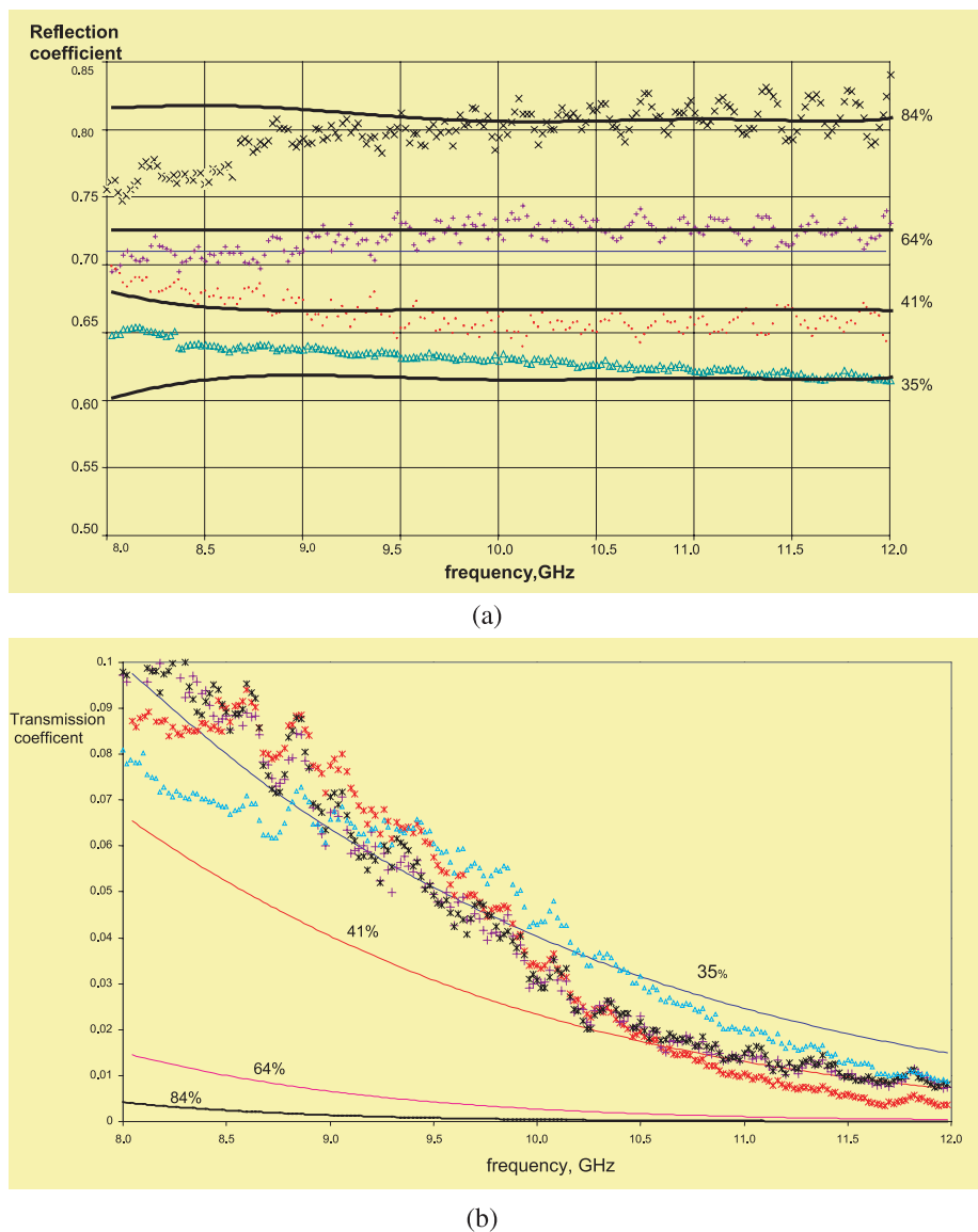
Fig. 3. Variation in (a) reflection coefficient (b) transmission coefficient with frequency. ( \times 84% + 64%041% \Delta 35%)
