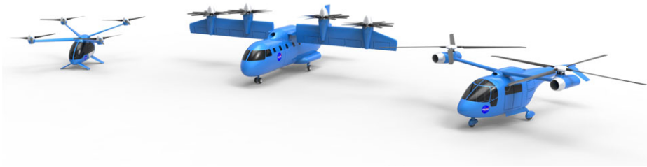
Figure 3. Concept aircraft: single-passenger quadrotor with electric propulsion, 15-passenger tiltwing with turboelectric propulsion, and 6-passenger side-by-side helicopter with hybrid [4].
