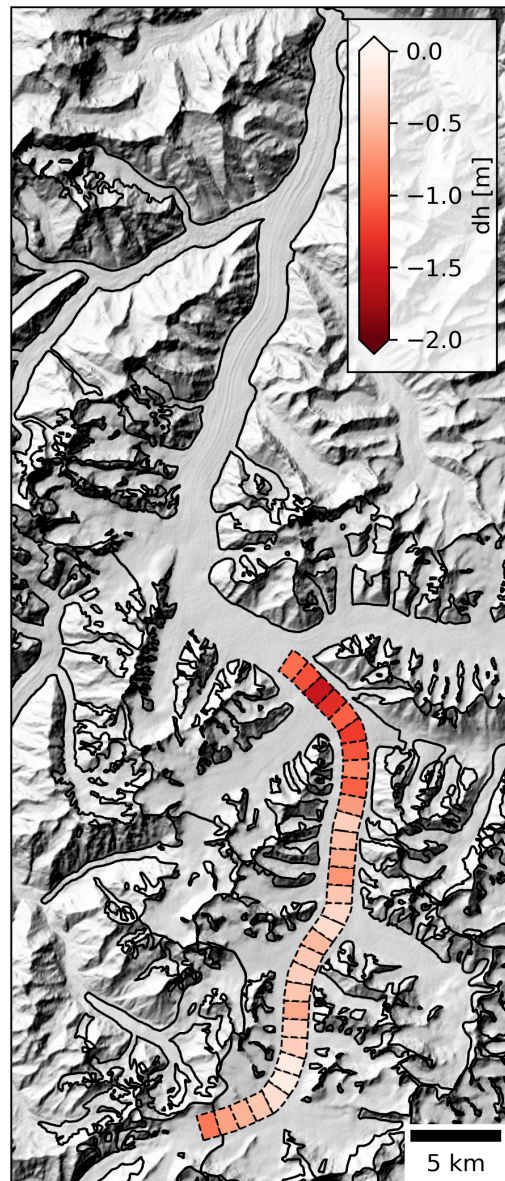
Fig. A4. Elevation difference between the Pléiades DEM of 22-23 September 2019 and the Pléiades DEM of 1-2 August 2019 that is used for the seasonal correction of GNSS data.
