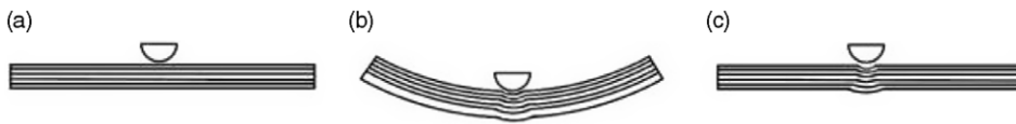
Figure 17. Impact response mechanism of Vectran/MTM57 laminates under low velocity impact loads (a) Before impact (b) During impact (c) After impact.
