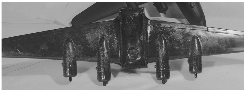
Figure 1. World War II era photograph of a unpainted wing section. Injection point on fuselage and flow lines visible on surface indicate potential stress points and sites of future shrinkage and cracking.
