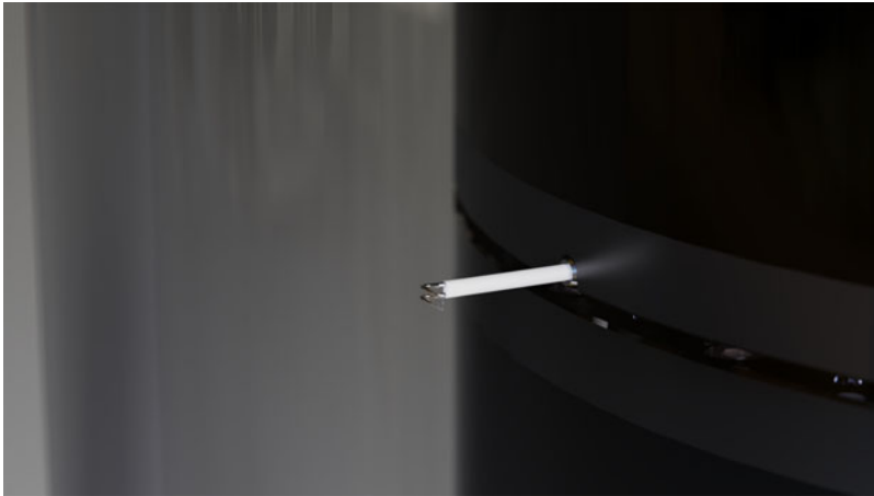
Figure 4. A volumetric rendering of the CTA probe mounted on the inner cylinder in the flying hot-wire configuration. The probe causes minimal disturbance on the azimuthal flow as its blockage area is only \approx 0.1\% of the cross-sectional flow area (in the axial–radial plane).
