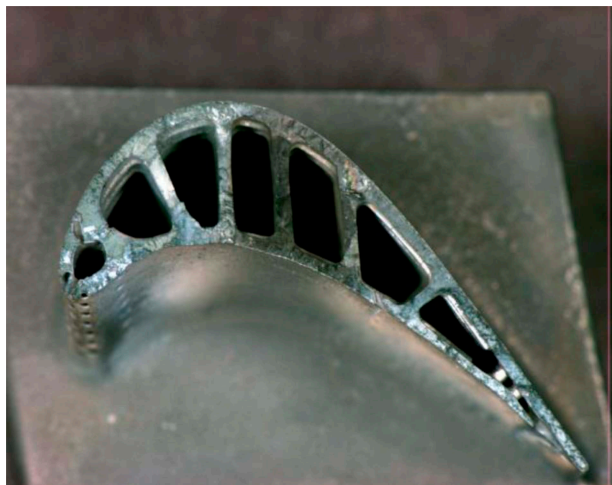
Figure 1. The fracture surface of the failed HPT blade. The dark region over the 4 th and 5 th web from the leading edge is oxidation cracking.
