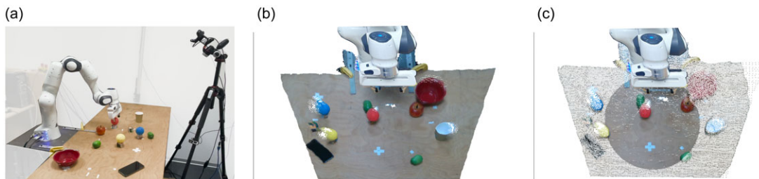
Figure 14. Teleoperation experimental setup, a virtual model of the robot, and point clouds streamed in FREF and F2 experimental conditions.
