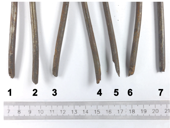
Figure 2. Disassembled strand, wires 1-6 circumferential wires. Wire 7 from the center failed by cup and cone fracture.
