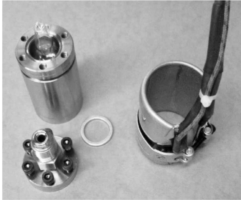
Figure 4 Cs oven and band heater. The new oven mates with the smaller of the 2 VCR nuts shown at the top of the NEC oven assembly in Figure 1.
