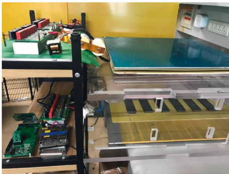
FIGURE 9: Experimental setup for wireless power transfer under inhomogeneous winding.
