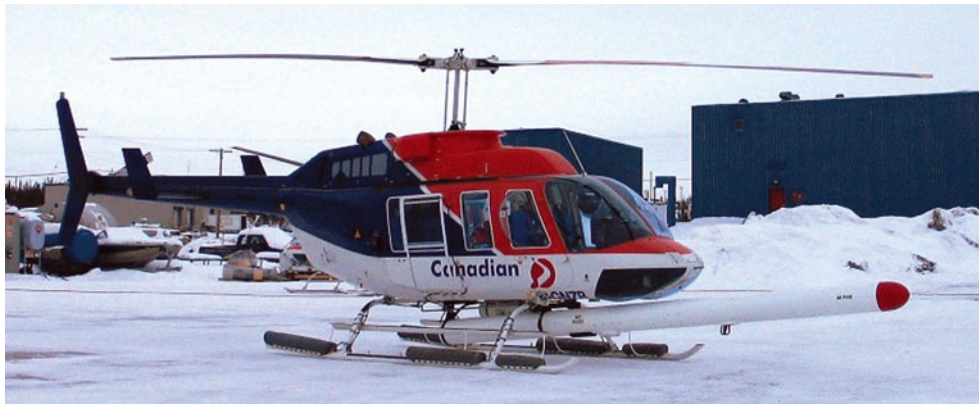
Fig. 1. Canadian Helicopter Ltd Bell 206L helicopter showing the fix-mounted sensor equipment. The EM sensor is located in the outer section and the video-laser in the middle section of the cigar-shaped mount.
