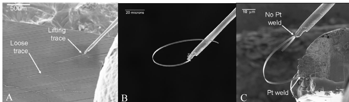
Fig. 2. A. Lift-off of 0.65 wide micron copper trace from test wafer. B. Extracted copper trace. C. One end of trace attached to grid and free end held by static charge ready to span air gap.
