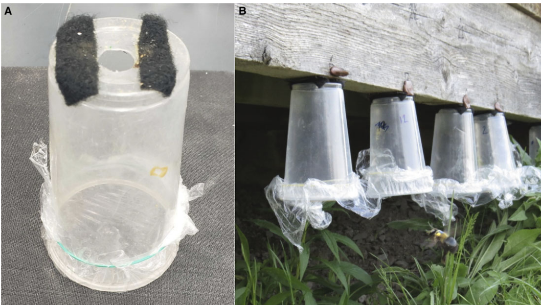
Fig. 1. Cup trap used to capture bees arriving and departing from nest entrances: A , each cup has a hole cut in the base, two strips of Velcro on the base, and an elastic band and cellophane to cover the open side of the cup; B , cups were attached over each nest entrance.
