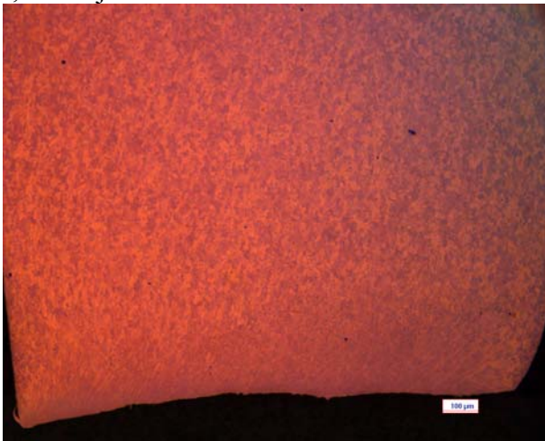
Fig. 3. CP Ti Sheared, as polished viewed in polarized light and sensitive tint, 5X objective
