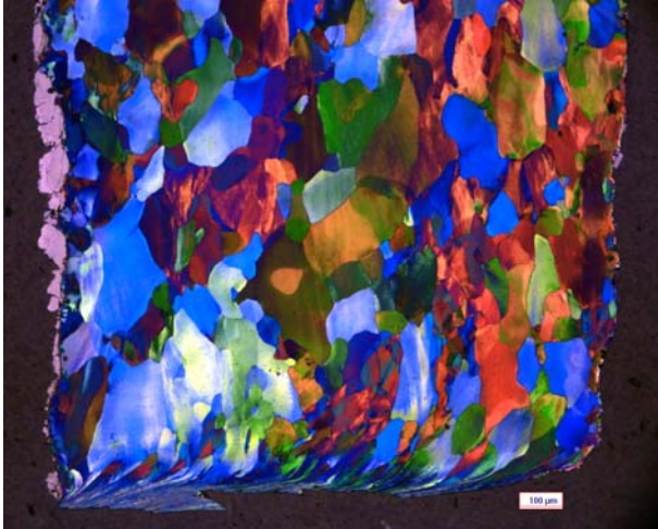
Fig. 1. 99.98 Fe sheared, etched with Klemm's I, 5X objective.
