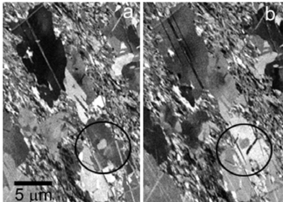
FIG. 1. Ultrafine grained Cu imaged in the CL mode at 2 keV (primary energy 6 keV): untitled sample (a), sample tilted to 1.4° (electron impact at 2.4°) (b); encircled area of inversions in contrast of twins and subgrains.
