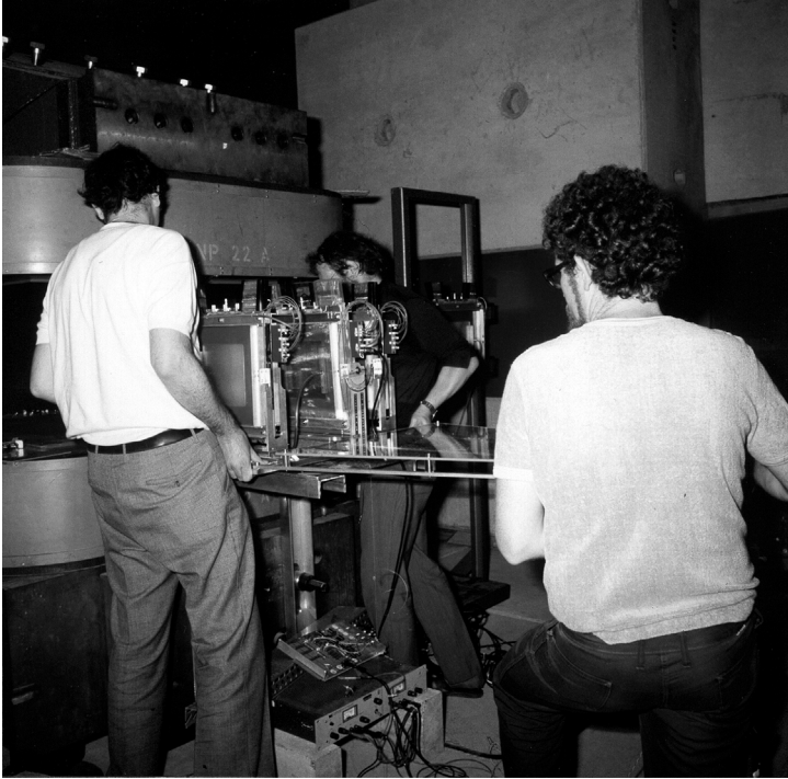
Figure 1.9 Guy Schultz (left) and Amos Breskin (right) inserting a set of high accuracy drift chambers in a magnet. Picture CERN (1972).
