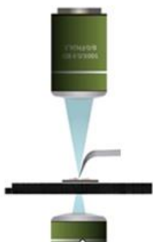
Figure 1. Probe design with open access of the electrical probe to optical and electron beams
