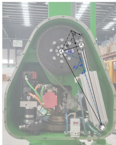
Figure 4. Compensation torque analysis of joint 3.
