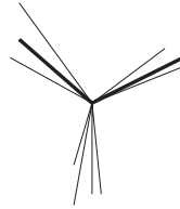
Fig. 12.18. Three-jet configuration with registered particles (thick lines) in two of the jets. The line lengths indicate momenta.
