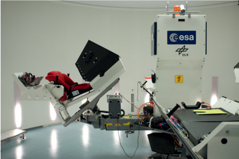
Figure 22 A human centrifuge at the DLR in Cologne. The centrifuge rotates about a vertical axis with observers are either supine – the arm on the right-hand side – or are seated in a chair that can be positioned at a range of orientations. Displays and other devices rotate with the observer.
