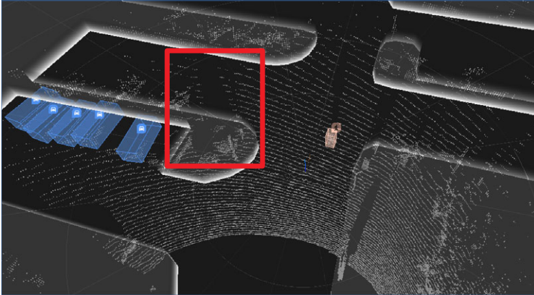
Figure 7. Road side scenario. The white edges represents a virtual wall of the ROI, blue boxes denotes the vehicles, and orange box is a pedestrian. The red box area denotes an occlusion caused by a tree.
